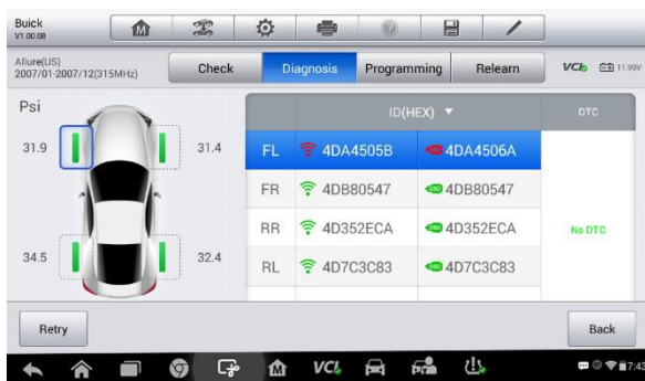
Figure 6-13 Sample No DTC Screen
