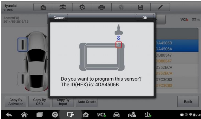
Figure 6-18 Sample Copy by Activation Confirmation Screen
