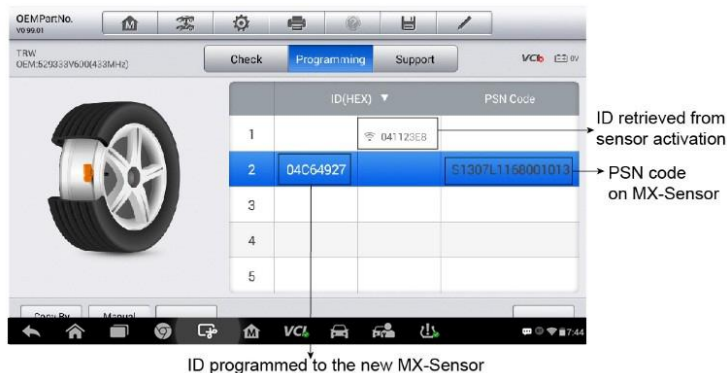
Figure 6-34 Sample Programming Screen via OEM Part No.
