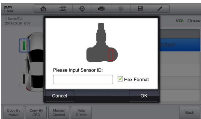
Figure 6-22 Sample Copy by Input Screen
