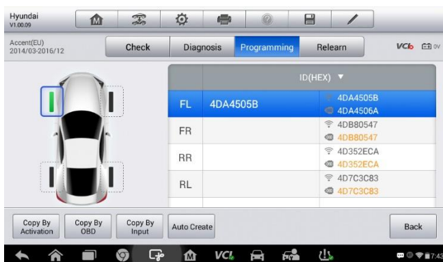
Figure 6-20 Sample Copy by Activation Complete Screen
